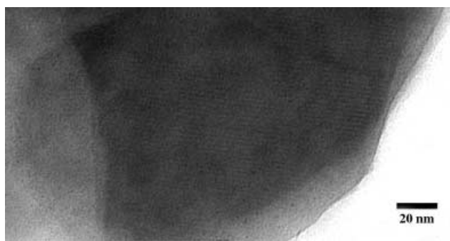
Figure 6. TEM image of the [\text{Ni}_3\text{P}_3\text{S}_{12}]^{3-}/\text{DiC}_{12}\text{DA} complex deposited on a perforated carbon-film copper grid from chloroform at room temperature.
